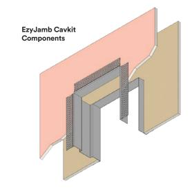
EZ Concept Cavkit is a **trim kit only** and does not include the cavity sliding door, frame or track. Cavkit is designed to suit most brands of cavity sliders. Cavkit standard components assumes the lining board is the same on both sides. Please contact EZ Concept if the lining boards are not equal thickness.
