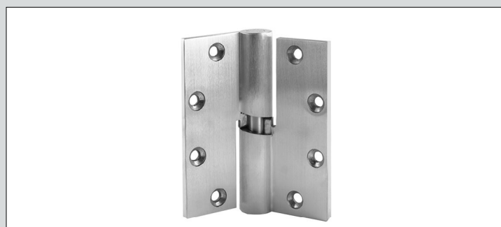
■ A9500 Cam Lift Hinge 5" x 4.5" Cam Lift Hinge 5/16" of lift, can hold up to 900lbs.
