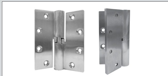
■ A9500 Cam Lift Hinge 5" x 4.5" Cam Lift Hinge 5/16" of lift, can hold up to 900lbs.
